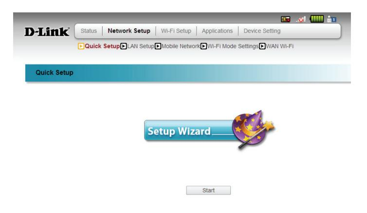
If you don't have a SIM card inserted into the DWR-932, the screen shown to the right will be displayed. You will need to power off the device, insert a SIM, and restart the wizard to complete the quick setup process.
