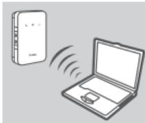
1. Use your PC's wireless adapter to connect to the **dlink\_DWR-932\_xxxx** wireless network. The wireless network name (SSID) and password are printed on the label under the battery.
