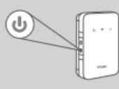
6. Press and hold the power button for four seconds to turn on the device. Once the power LED icon lights up solid green you may proceed with configuration.
